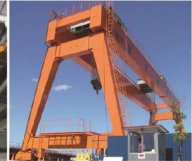
2010 Airport Metro Line 260 Tons Gantry Crane Project
